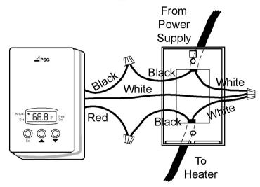
Attach wires per diagram above.
